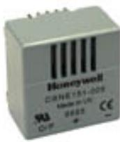
**CSN Series closed loop current sensor, measures ac, dc or impulse current, 25 amp-turns nominal,  $\pm 43$  amp-turns range, high temperature, potted, 1000 turn**
