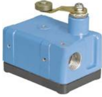
Enclosed Switch Series OP: Side Rotary, Fixed lever length with steel roller, 1NO 1NC Snap Action SPDT, CW actuation, High capacity
