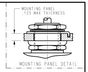
HARDWARE FURNISHED ASSEMBLED WITH SWITCH OR IN PACKET PER MIL-PRF-8805
