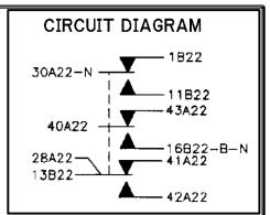
5 - SWITCH CURRENT LEVELS SHALL NOT BE MORE THAN 100 MILLIAMPS AT 28 VDC
