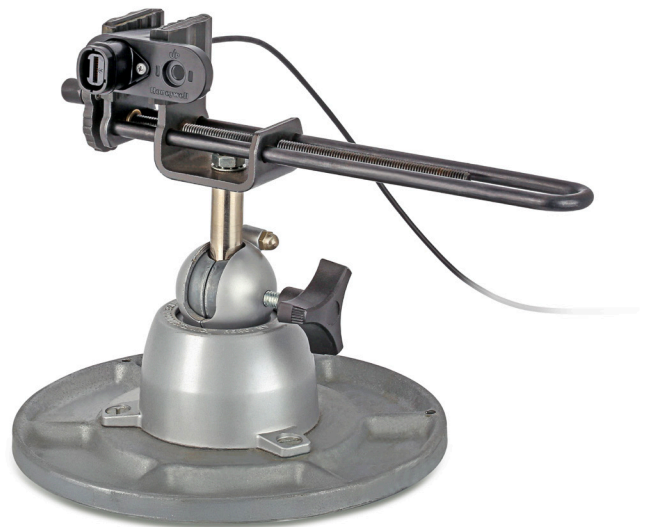
Figure 4. Mounted Using a Vice
