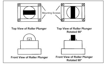
The head can be rotated by carefully removing the four combination head screws holding the head in position. Carefully remove the head assembly and rotate to the desired position. Replace the head assembly and tighten the mounting screws. Ensure that the head is properly located. Hand test the actuator to ensure that the switch functions and the actuator moves freely (sticking can occur if material has been deposited inside the drive train whilst the head assembly was removed).
