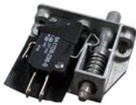
AC Series Door Switch, Single Pole Double Throw Circuitry, 5 A at 250 Vac, Rod Actuator, Silver Contacts, Quick Connect Termination
