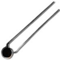
143 Series, 5,08 mm [0.2 in] disc thermistor with leads, 1,000 Ohm resistance, \pm 10.0\% tolerance, 25/85 BETA = 3974
