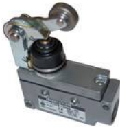
Enclosed Switches Series E7: Top Roller Arm Actuator, Adjustable with Steel Roller; 1NC 1NO SPDT Snap Action; PG13,5 conduit
