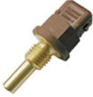
ES120 Series immersion temperature probe, NTC, 2,000 Ohm,  $\pm 5.0\%$  tolerance, 20 °C [68 °F] accuracy, brass, threaded body (M12x1.5), overmolded connector/2 Pin MINI TIMER
