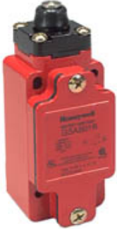
GSS Series , Safety Lim it Switch, 1NC/1NO Direct Opening, Snap Action, Top Pin Plunger, 20 mm , EN50041, Zinc Die-cast, Silver Contacts
