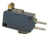
V-Basic Standard V15 Series, 5 A, roller lever, 6,35 mm x 0,80 mm quick connect terminals, SPDT, 100 gf [0,98 N], gold-plated contacts
