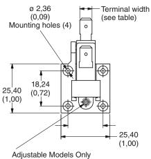
Adjustable Models Only Adjustment screw 1,98mm (,078) Hex socket – clockwise to increase actuation point, counterclockwise to decrease actuation point
