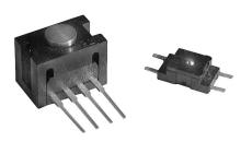
The FS Series Force Sensors provide precise, reliable force sensing performance in a compact commercial grade package. The sensor features a proven sensing technology that utilizes a specialized piezoresistive micro-machined silicon sensing element. The low power, unamplified, noncompensated Wheatstone bridge circuit design provides inherently stable mV outputs over the force range.
