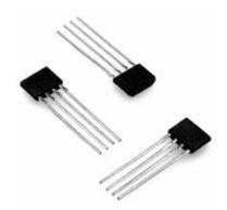
The SS42R Series is a Bipolar Latching Hall IC with a pair of complementary push/pull outputs. A dual Hall element is used to offset stress induced noise and drift. The operate and release points are laser trimmed to insure near-zero symmetry. The robust outputs are capable of sourcing up to 6.4 mA and sinking up to 4.4 mA. The device contains inherent reverse polarity protection up to the full power supply rating.
