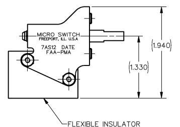
2 - SWITCH WILL PERFORM SATISFACTORILY IN TEMPERATURES TO MINUS 20°F 3 - CATALOG LISTING, DATE OF MANUFACTURE AND FAA-PMA IS MARKED ON BRACKET
