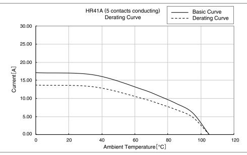
Note 2 : The derating curve is derived from the basic curve multiplied by the derating factor of 0.8.
