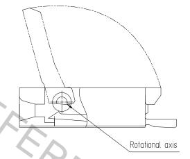
3. Please do not push downwards to the Actuator with more than 0.5N force, as shown below. Otherwise, the Actuator may fall off or be damaged.
