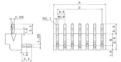
Note: The kink process is alternately performed in optional directions.
