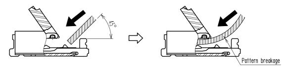
3. Do not rotate the actuator when FPC TAB is on Metal Fittings.
