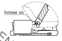
3. The actuator will not open more than 125°. Do not apply any force backward beyond this point. Otherwise, the actuator may come off or break.
