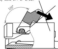
4. Move the actuator at approximately the center. Otherwise, the actuator may come off or break.
