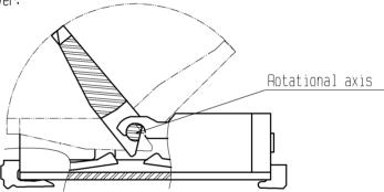
3. The lock lever will not open more than 135°. Do not apply any force backward beyond this point. Otherwise, the lock lever may come off or break.
