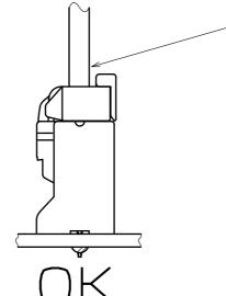
No stress concentration: No cable bending close to connector
