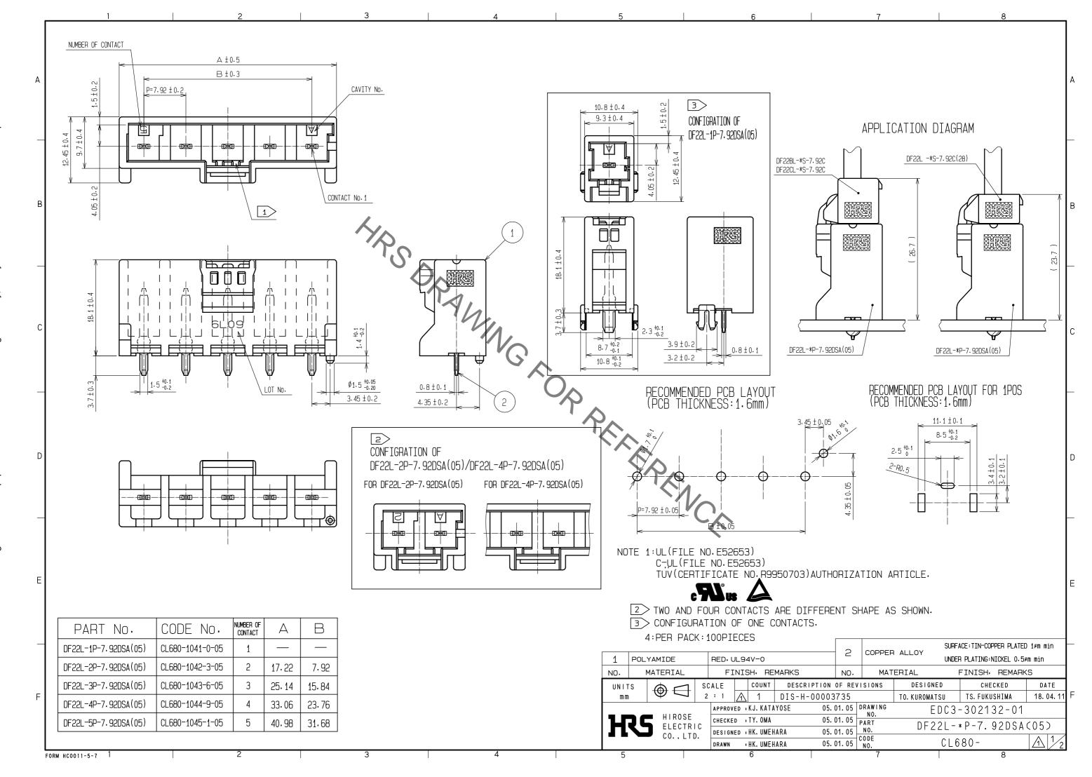
$\triangle$ Precoutions ◆Notification for Insertion Extraction 1) Please insert(extract) the crimping socket straight to the mating connector. Insertion(extraction) at tilted angles applies load concentration to the connetor end and may cause deformation (at connection area, socket and header case, etc). There is firing risk using this kind of defomed connector. Insertion(Extraction) Insert/extract vertically Insertion
