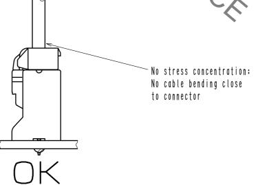
2) When applying load to connector end, please use the retainer for reducing the stress affection on the connector. Retainer shall be installed after inserted crimping contact completely. It might be impossible to insert it when terminal installation is incompleted.
