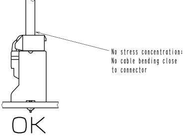
2) Since this product uses thick wires, a larger load is applied to the connector when inserting/extracting or routing the wires. Please use a retainer to reduce the load on the connector.
