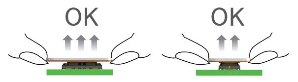
If difficult to remove, extract the connector diagonally in the direction of the pitch. Note that removal from the widthwise side will apply a large load to the contacts. When removing from the width direction, pull the end of the FPC in the upward direction. (When a force is applied in the horizontal direction, a large load is applied to the contact.)
