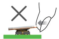
If the FPC does not have sufficient rigidity, solder stripping or connector breakage may occur. Please use it after checking the repetitive operation with a flexible board in advance, such as during a trial manufacture run (Left diagram).
