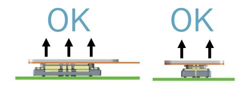
2. If difficult to remove, extract the connector diagonally in the direction of the pitch. Note that removal from the widthwise side will apply a large load to the contacts. When removing from the width direction, pull the end of the FPC in the upward direction. (When a force is applied in the horizontal direction, a large load is applied to the contact.)
