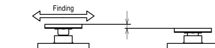
(2) WHEN GUIDING, THE CONNECTORS ARE ALIGNED PARALLEL TO EACH OTHER, WITH LONGITUDINAL AND LATERAL MOVEMENTS RESTRICTED. MATE THEM PROPERLY BY APPLYING FORCE IN THIS CONDITION.
