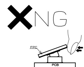
(3) IF THE FPC IS NOT RIGID, THE CONNECTOR CAN BE BROKEN. PLEASE CHECK THE ACTION OF THE FPC TO BE USED REPEATEDLY AT THE TIME OF TRIAL PRODUCTION. BE CAREFUL TO UN-MATE THEM FROM THE PITCH DIRECTION.
