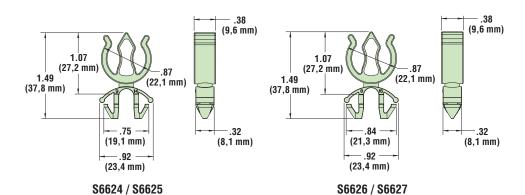
Material Black Heat Stable / UV Stable Nylon Temperature Range -4°F (-20°C) to 185°F (85°C)
