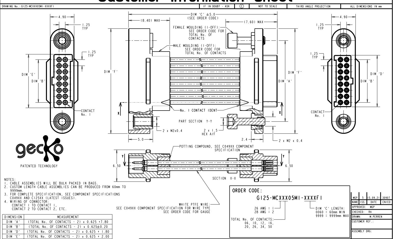
DIM 'F' (TOTAL No. OF CONTACTS - 2) x 0.625 + 12.7 FXAMPLE PART No. 12 CONTACT CONNECTORS WITH 150mm OF 26AWG WIRE = G125-MC11205M1-0150F1
