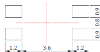
Figure 1. IN-P32TRRRGB Solder Pattern
