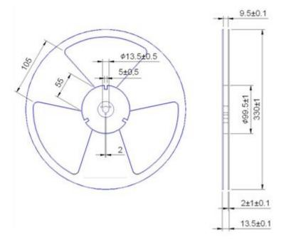
Unit: mm Tolerance: +/-0.15mm
