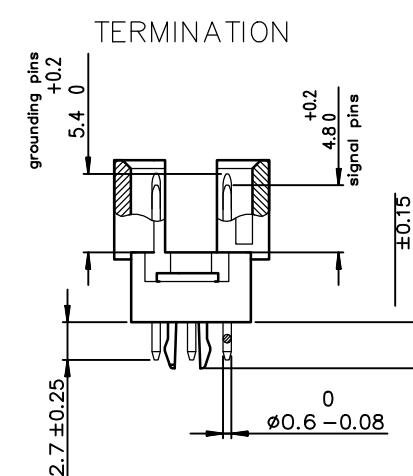
SPECIFICATION 113 = 8 grounding pins in position :
