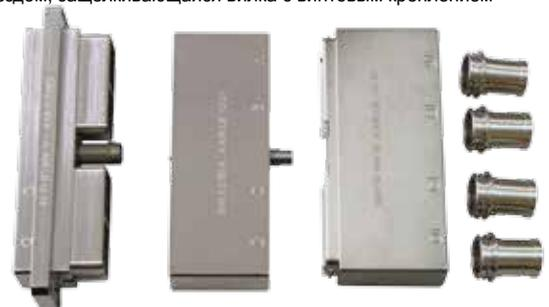
*Metallic SIM Connector with Nickel plating, shells for 4 modules with Short Flanged receptacle, Clicker Nut Plug and Plug Cover with Chimneys*
