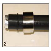
Step 2: Slide backnut and gasket onto cable. Trim and remove 13/32" of the cable jacket. NOTE: Do not cut the outer drain wire.
