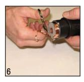
**Step 7:** Trim the copper tape so that it is even with the core.
