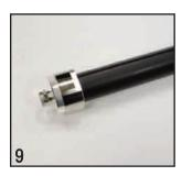
Step 10: Using 2.0" box wrenches, fully tighten down the connector until snug. Go one-quarter turn to completely tighten. NOTE: It is recommended to use an additional stress boot at the cable to connector interface. A shrink boot, silicone tape or strong electrical tape will add strength.
