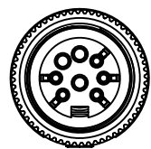
AISG 8-pin female interface with 5 loaded contacts
