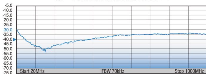
S11 TYPICAL RETURN LOSS (dB)
