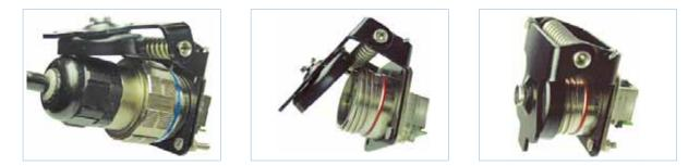
This Self Closing cap automatically protects the RJF TV square flange receptacle (MIL-DTL-38999 type), protecting your system from dust and water projection. A spring automatically closes the upper part of the cap when the RJF TV plug is removed from the receptacle.
