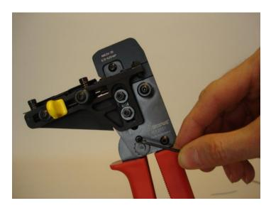
Be sure that the tool is open. Adjust the crimping height by means of the crimping height adjustment key. Attention! A miss adjusted crimping height can damage the tool.
