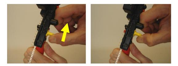
Feed a terminal into the crimping area of the hand tool.
