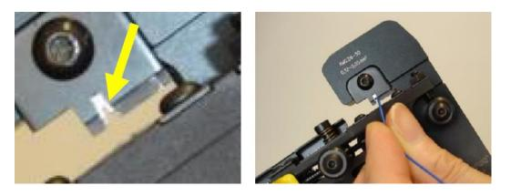
While keeping carefully the wire in position, close the handles until the ratchet releases.
