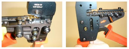
As shown on the picture, insert the strands of a stripped and straightened wire into the slot of the wire positioner. The insulation of the wire should be pouched to the surface of the wire positioner.
