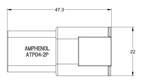
KIT, ATP SERIES, 2 POSITION, RECEPTACLE, CONTACTS, & WEDGELOCK
