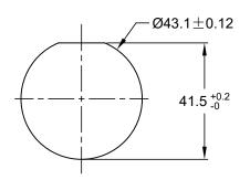
RECOMMENDED PANEL **MOUNTING HOLE** RECOMMENDED PANEL THICKNESS:1.6 TO 4.7MM
