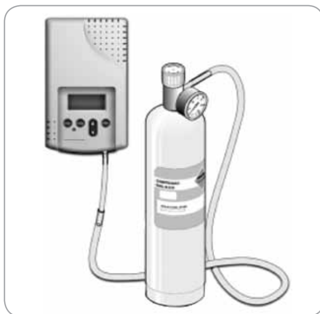
The illustration shows the complete set-up for calibrating a sensor with display.
