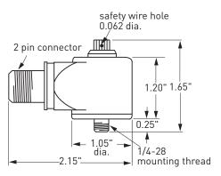
Accessories supplied: #12105-01 captive socket head (metric mounting available); calibration data (level 3)
