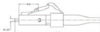
LC Duplex Connector with 900μm Boot
