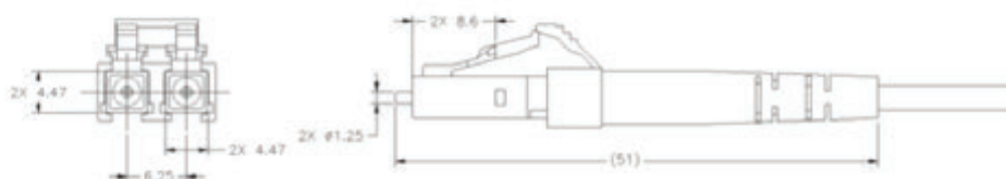
LC Duplex Connector with 1.6/2.0mm Boots
