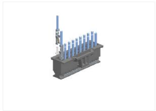
Insert the terminals into the active latch housing.
