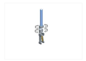
Crimp the terminal onto the wire.
