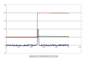
The chart to the left shows the difference between the response of an RMS transmitter, a peak transmitter, and the Wilcoxon true peak transmitter. The RMS and peak outputs change very little as a result of the transient acceleration pulse. However, the true peak signal actually "captures" the pulse level accurately.
