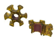
Power Feeder Spacers separate and provide a constant spacing between the power feeders. The custom design of this product allows a six degree rotation on the power feeder bundle and doesn't fight against the natural flow of the cable. It is designed to sit within Omega Clamps which can be used as anchor points.
