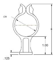
Amphenol Pcd's Jig Board Clamps are made for pre-installation wire harness assembly. Made of Acetal, our durable clamps maintain their original shape after continuous use and their smooth edges diminish wear on the harnesses as they are being assembled. Developed in multiple sizes, Amphenol Pcd's Jig Board Clamps can accommodate a wide range of cable diameters, while the one-piece design enables efficient inventory management.
