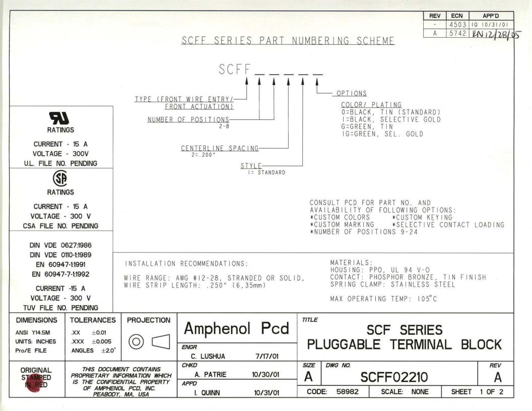
L=NUM OF POS X CL SPACING A=NUM OF POS X CL SPACING+.060
