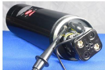
Figure 6: Probe connected to the test point pins
