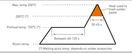
The recommended reflow profile is provided as a guideline. Optimal profile may differ due to oven type, assembly layout or other design or process variables.
